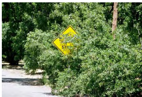
Figure 2. Signs need to be visible for traffic safety and driving convenience.
