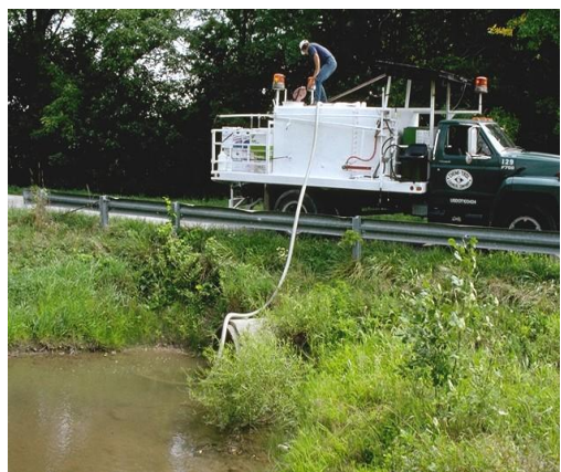
Figure 5. Chemical mixing should not occur adjacent to streams and creeks.
